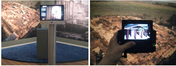
Figure 1: The revolvable display MovableScreen (left) and a UMPC (right) showing superimposed digital information layers on the two photographs in the back.
