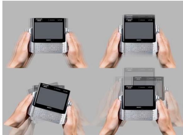
**Figure 4:** Interaction via motion determination
